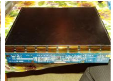
LCD panel electronics, column driver chips
