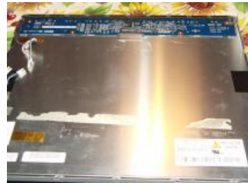
LCD panel, back, electronics exposed
