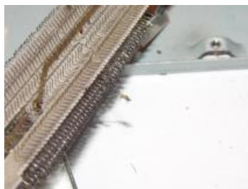
Broken wire, added brass
