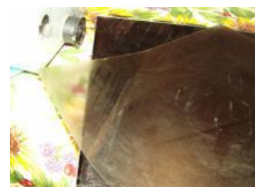
Unglued sheet, minor heat damage visible on the edge
