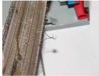
Broken wire, added brass and borax, foamed up
