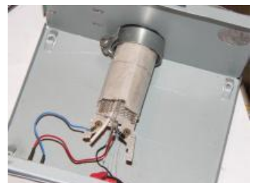
Inside view, heater mount
