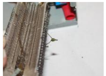
Broken wire, brazed together, before flux removal
