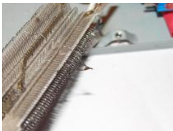
Broken wire, brazed together, before flux removal
